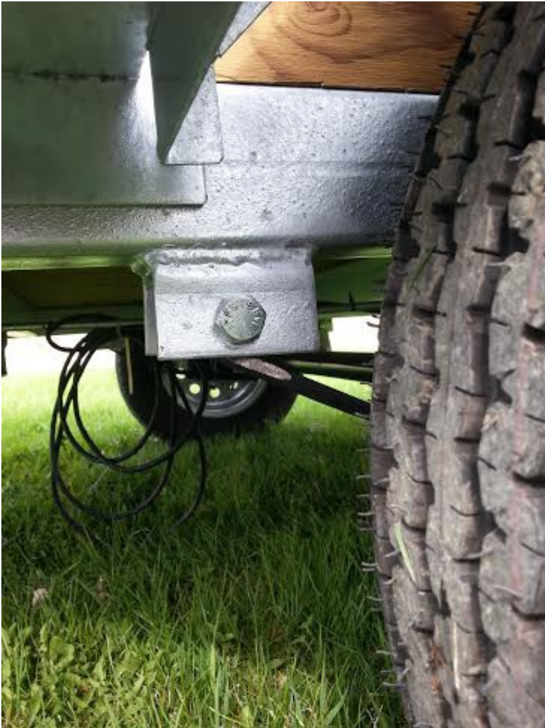
Shackle closest to the front of the trailer
